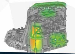
In order to control the quality of the key parts for the manufactory industry, we could use the PRINCE series handheld 3D scanner to obtain the geometry of the objects with ultra-detailed information, which could compare with the original CAD file. The inspector could easily find the deviation between the parts and CAD file or normal blue prints.
